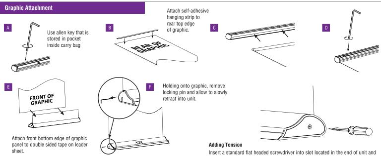
Note: To ensure a proper bond between graphic and double sided tape pressure must be applied. The adhesive should be allowed to cure for 24 hours before tension is applied.
